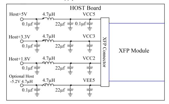
**Recommended High-speed Interface Circuit**
